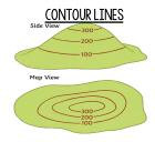
Contour lines are lines on a map which join up places of the same height. Everywhere along a contour line is the same height.
